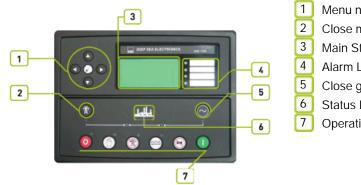
Menu navigation buttons Close mains button Main Status and instrumentation display Alarm LED's Close generator button
